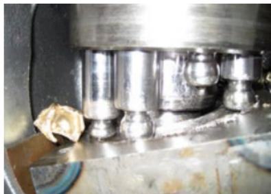
Axial pump damage due to cavitation
