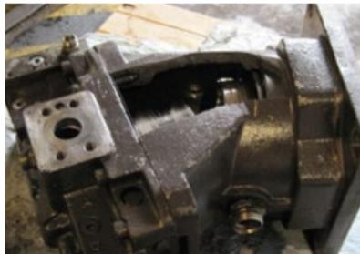
Defective hydraulic motor due to air in the system
