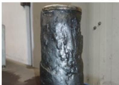
Contaminated system filter due to eroded hose inner layers
