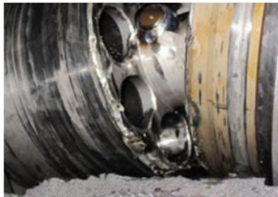
Defective axial piston pump due to oil contamination
